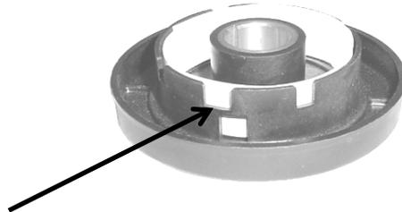
The thin area between the crank position and the cylinder position is the most common breakout location.
